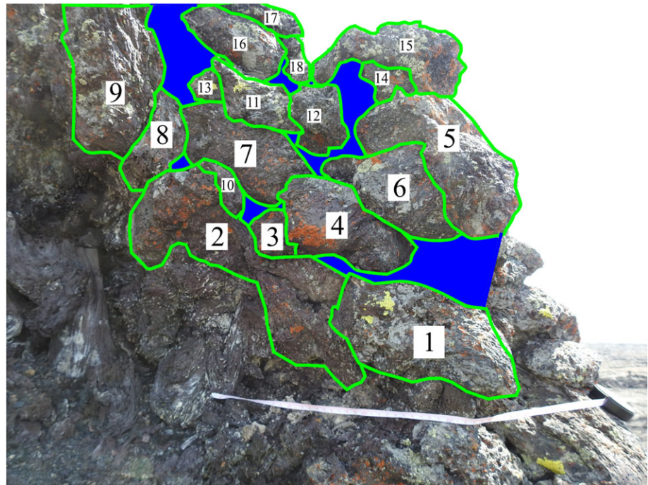
Figure 4. A photograph of HK17-01 showing the outlined, numbered clasts in green and void space between the clasts in blue. Cores of clasts that were not exposed were gently chiseled open so researchers could investigate the interior structure of each clast.
