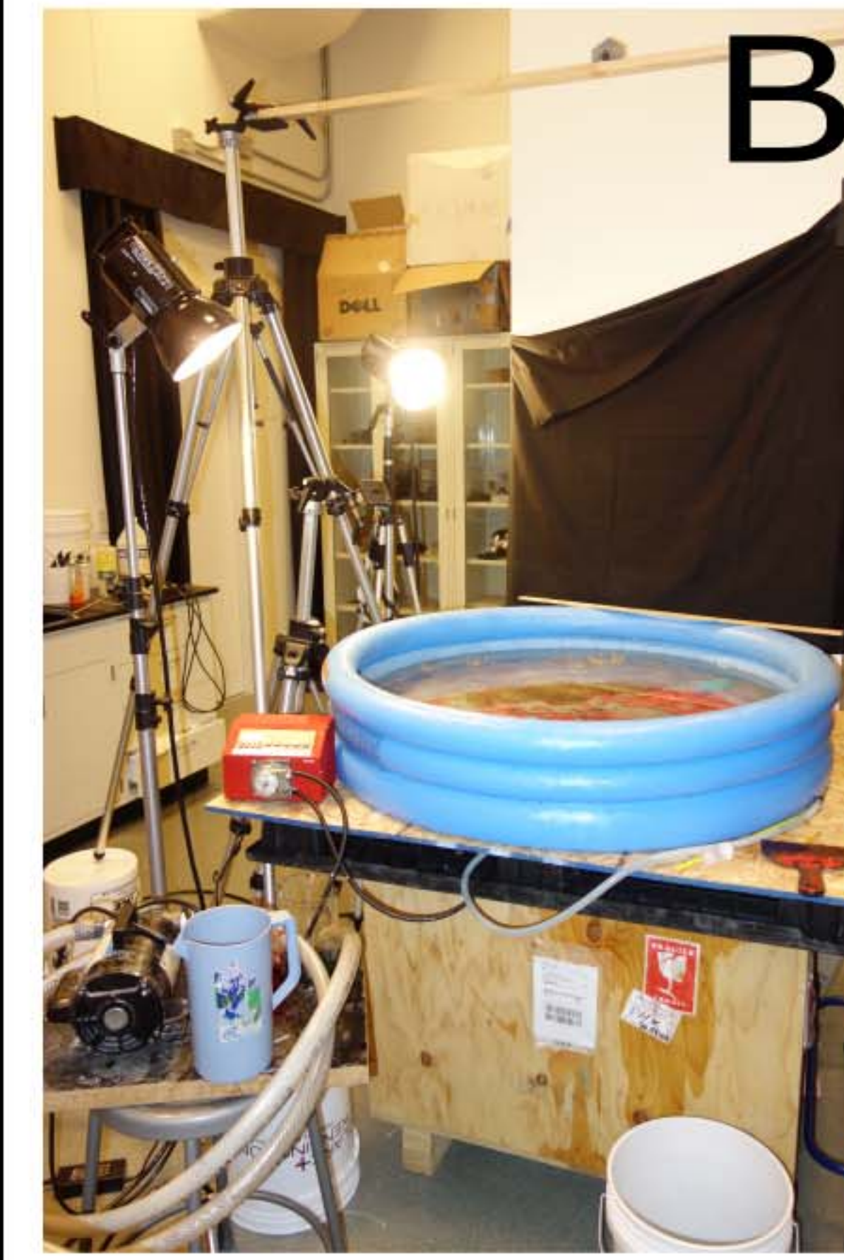
Figure 9. A large container to hold the water for the experiment can either be a clear-sided fish tank (A) or even an inflatable kiddie pool (B). With the clear-sided tank, non-water proof cameras can be used for all angles. The soft-sided kiddie pool requires water proof cameras, but the soft bottom can be molded to simulate topography.
