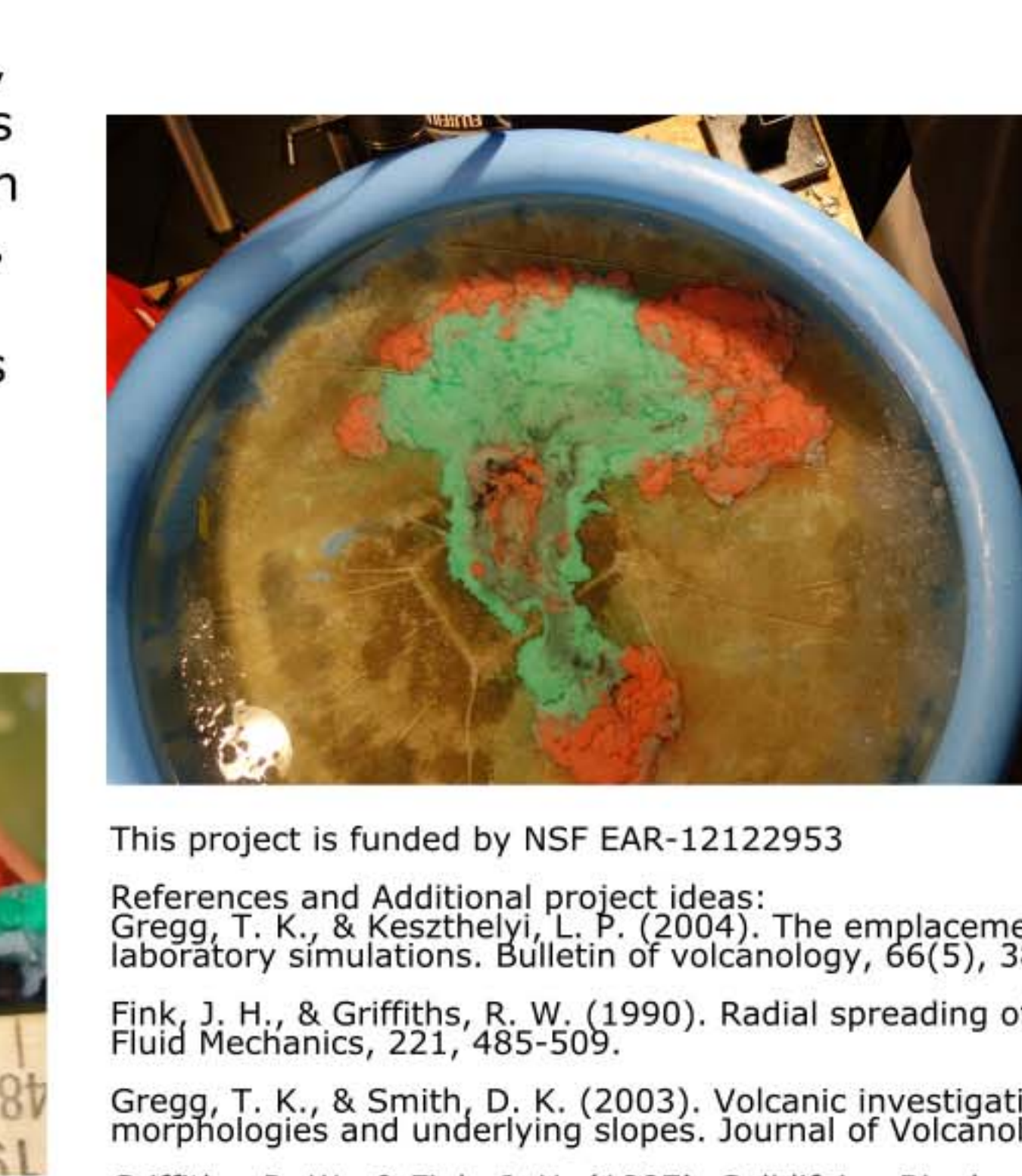
Figure 16. Wax dyed green, then red, then blue, records the formation and utilization of a lava tube within a flow. The observation of this phenomena allows students to hypothesize how lava, which cools very rapidly, can travel hundreds of miles.
