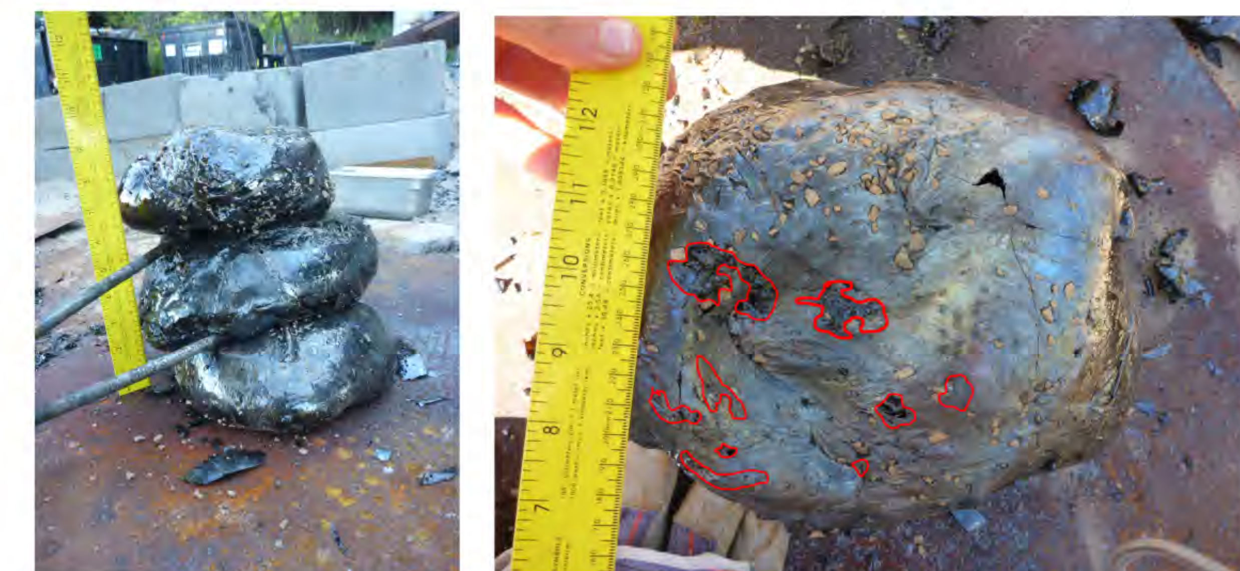
Figure 12. An experimental spatter pile sits with thermocouple probes extruding from the junctions between clasts on the left. After cooling, the piles are split apart for evaluation. One such evaluation is the percentage of surface area that was fused between the clasts, as seen on the right. Other measurements require clasts to be broken in half, like the size of vesicles and the thickness of the quench rind.
